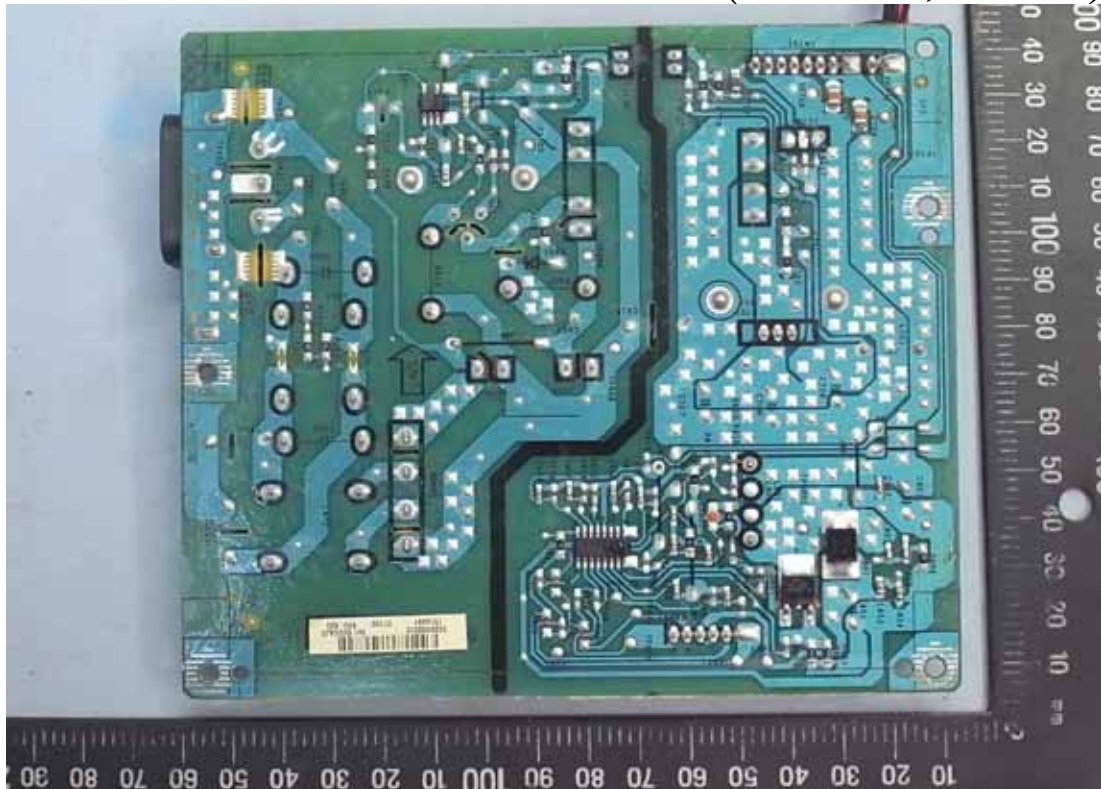
Figure 12 Internal View (Power Board, Back View)
