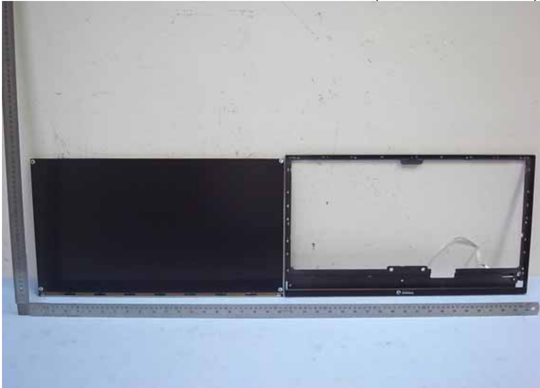
Figure 19 Internal View (Removed Front Frame)
