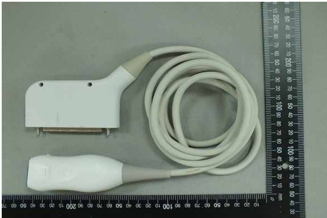
Transducer – 4 (Model No.: E94A, Supplier: Qisda Corporation)
