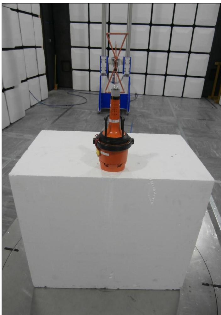
Figure 8 - Test Setup - 30 MHz to 1 GHz
