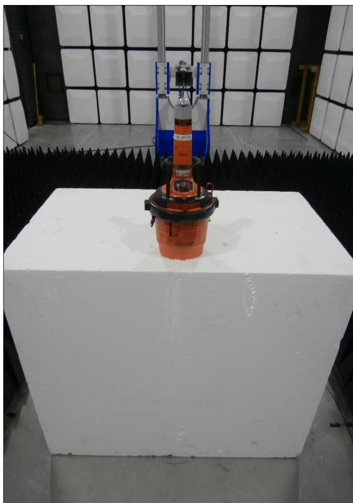
Figure 9 - Test Setup - 1 GHz to 2 GHz
