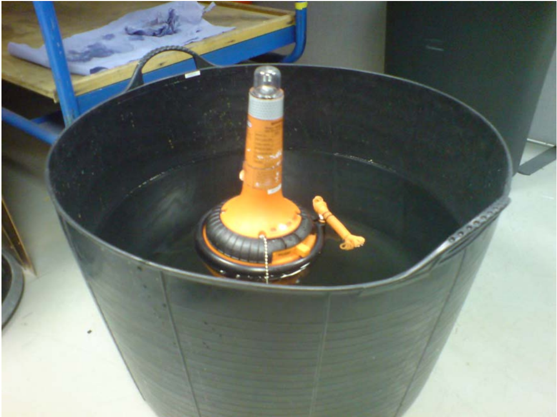
EUT Immersed In Fresh Water
