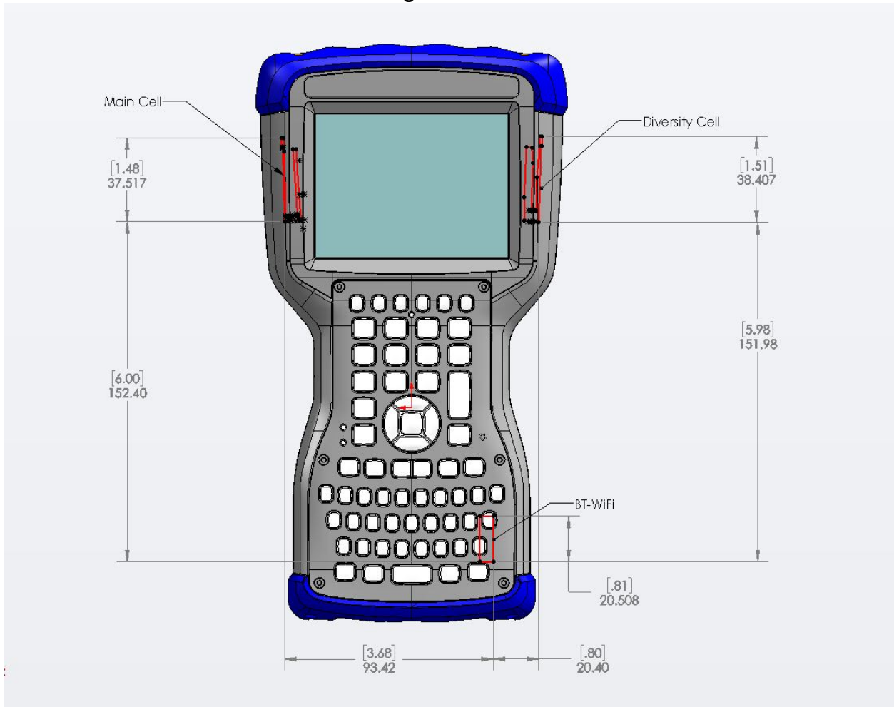
Figure 9.1 SAR Location Diagram of Antenna Distances
