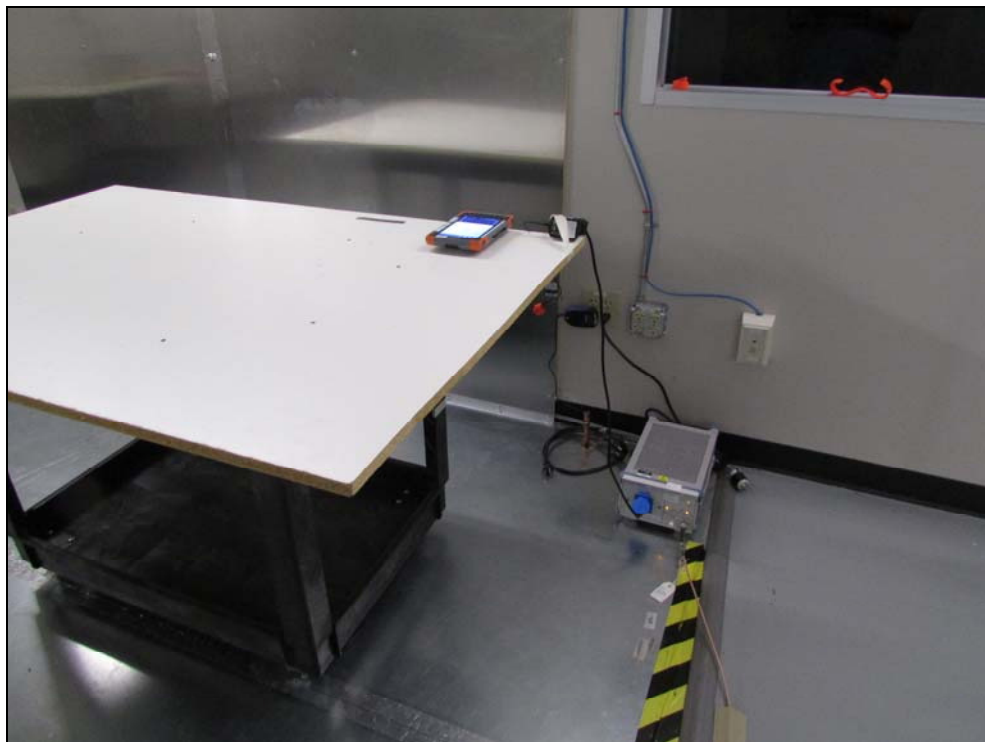
Figure 2: Power Line Conducted Emissions - Front
