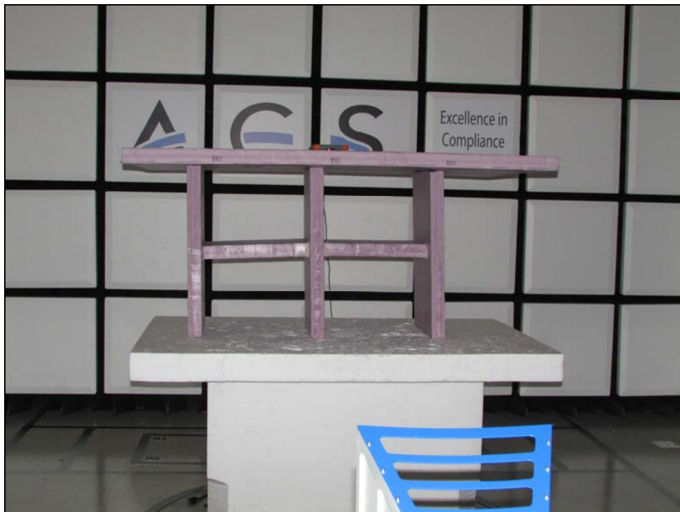
Figure 5: Radiated Spurious Emissions Above 1 GHz - Front
