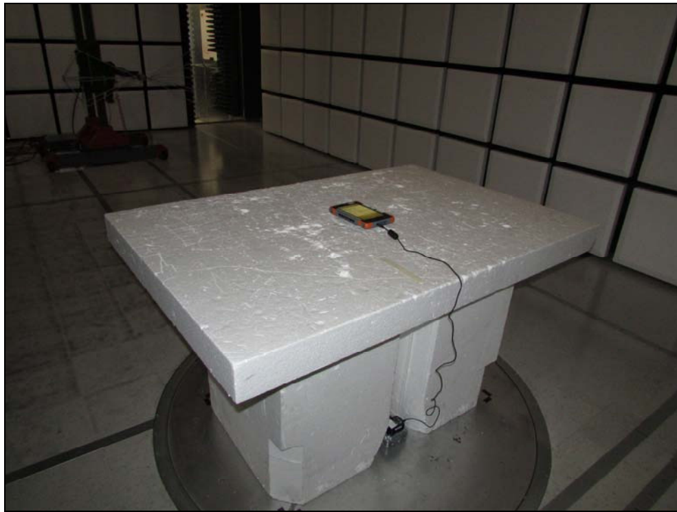
Figure 3: Radiated Spurious Emissions Below 1 GHz - Back
