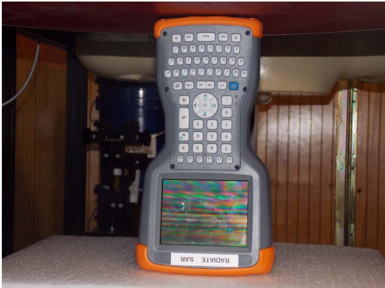
Test Position Bottom 0 mm Gap
