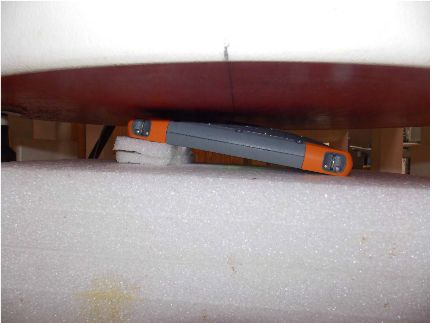
Test Position Back 0 mm Gap
