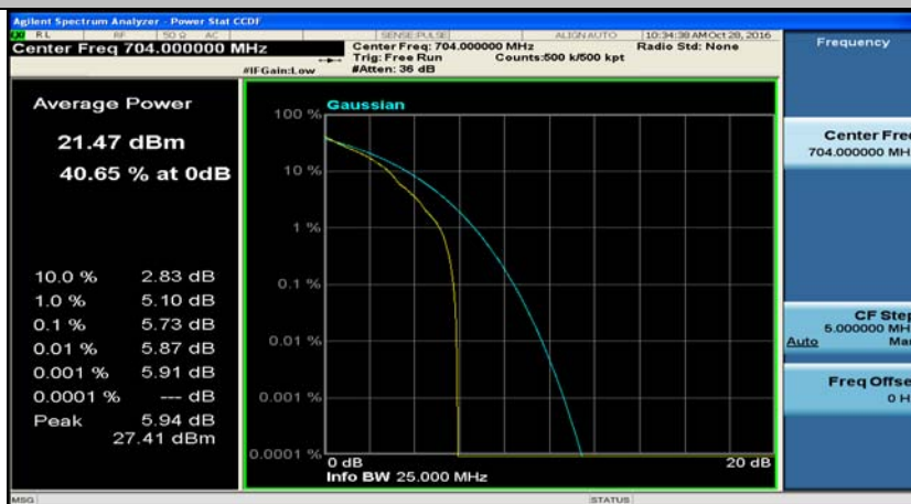
Channel Bandwidth: 10 MHz_LCH_QPSK_1RB#49
