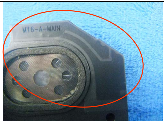
GSM/PCS/UMTS-FDD Antenna View
