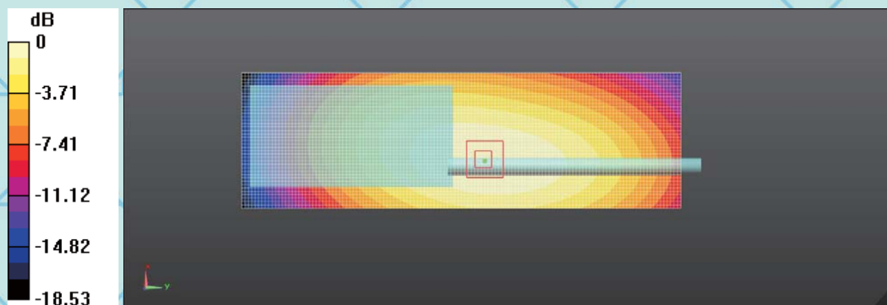
Plot 3: Body-worn for FM Modulation at 12.5KHz Channel Separation with A1, B1, BC1, AC1; Front towards Ground 450.50 MHz
