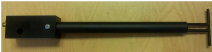
Figure 1 – MVG COMOSAR Validation Dipole
