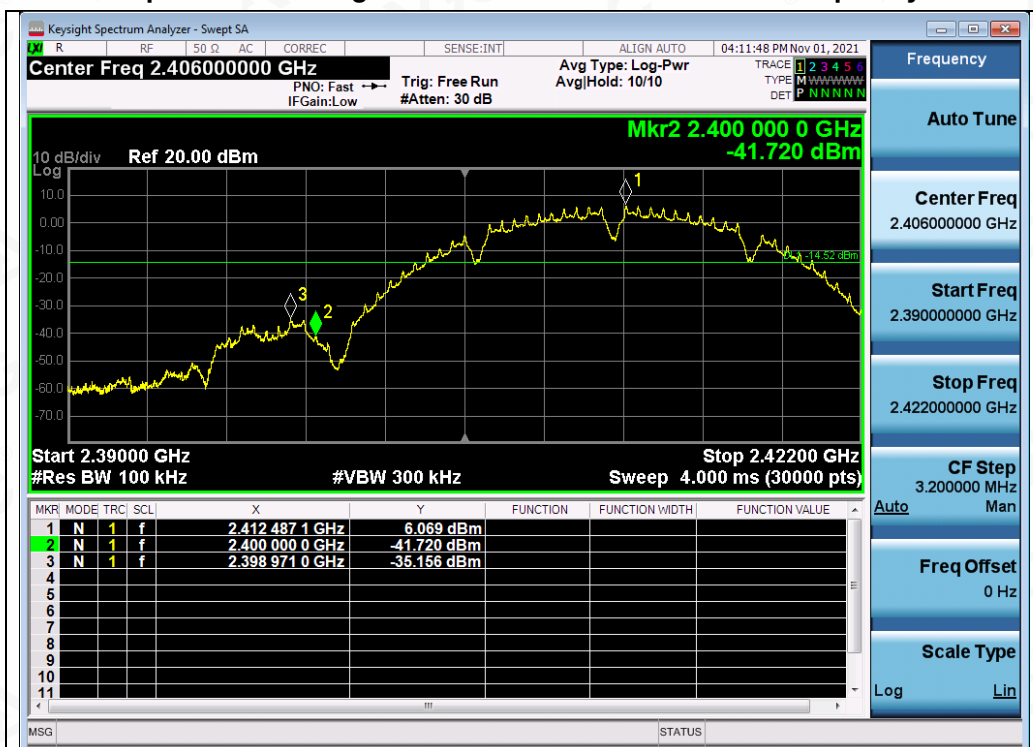
Test_Graph_802.11b_ANT1_2412_1Mbps_Lower Band Edge Emissions
