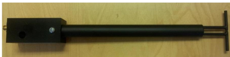
Figure 1 – MVG COMOSAR Validation Dipole
