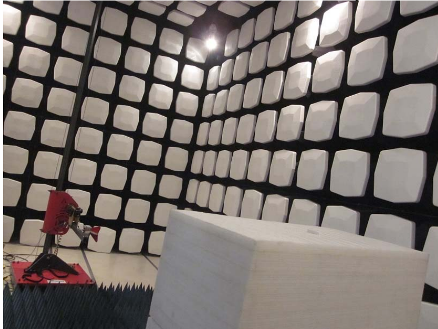
Measurement of Radiated Emission Test Set Up
