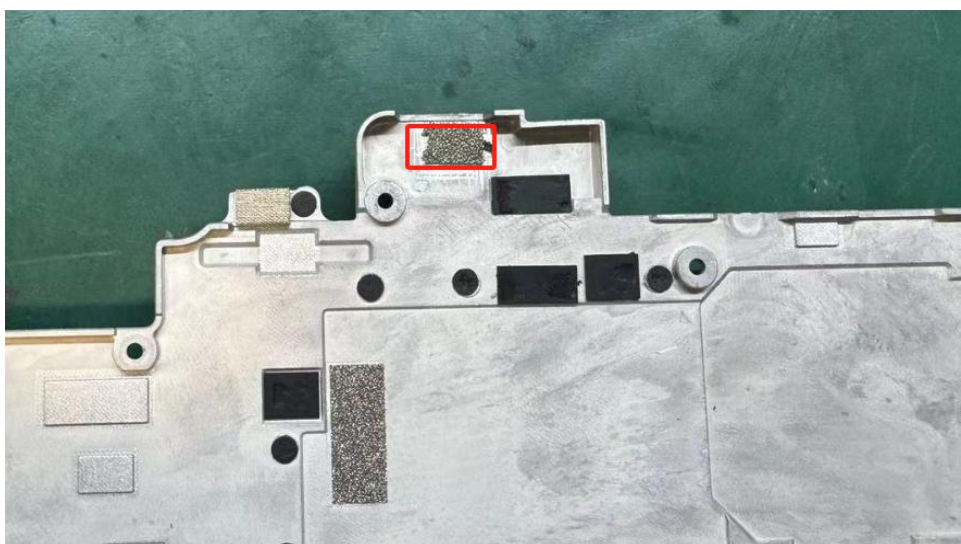
Add conductive sponge and small board USB grounding
