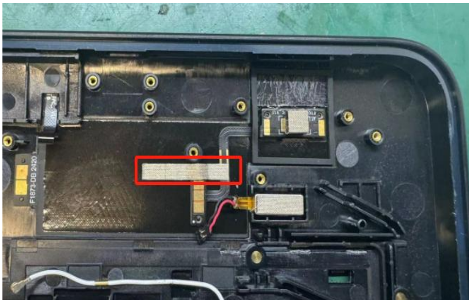
Speaker and motherboard grounding
