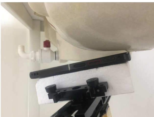
Left Tilted, Test Separation 0 mm
