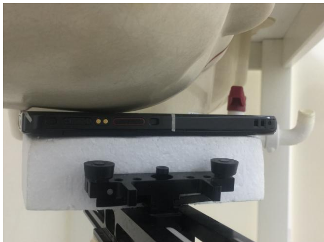
Right Cheek, Test Separation 0 mm
