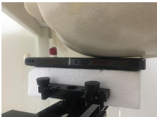
Left Cheek, Test Separation 0 mm
