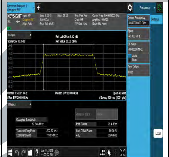
NTNV-n48-PC3-30-20-L-DFT-256QAM-Outer_Full-Ant1-PASS
