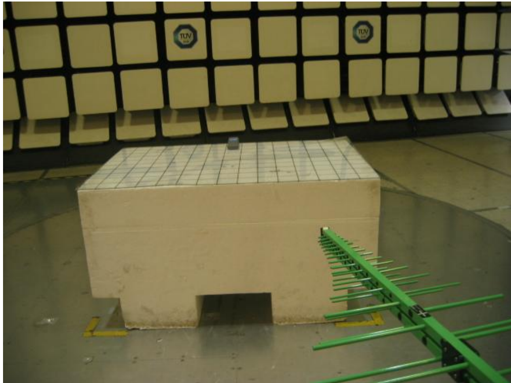
Radiated Emissions Test Setup (Front View)
