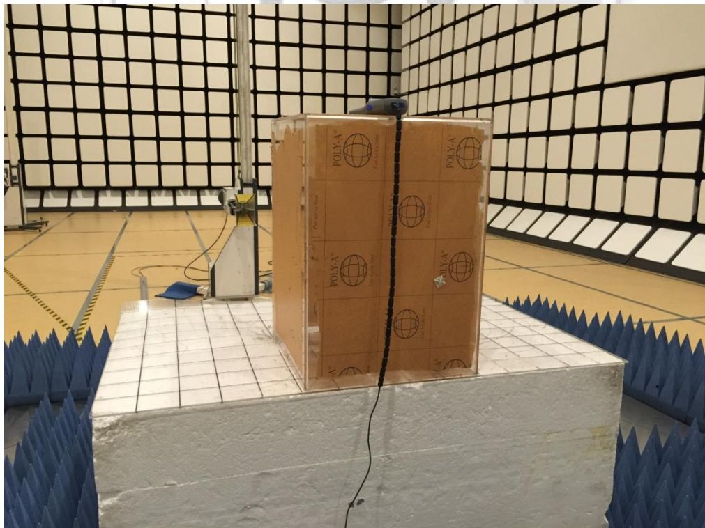
Radiated Emissions Test Setup (Rear View)
