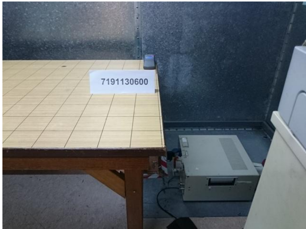
Conducted Emissions Test Setup (Front View)
