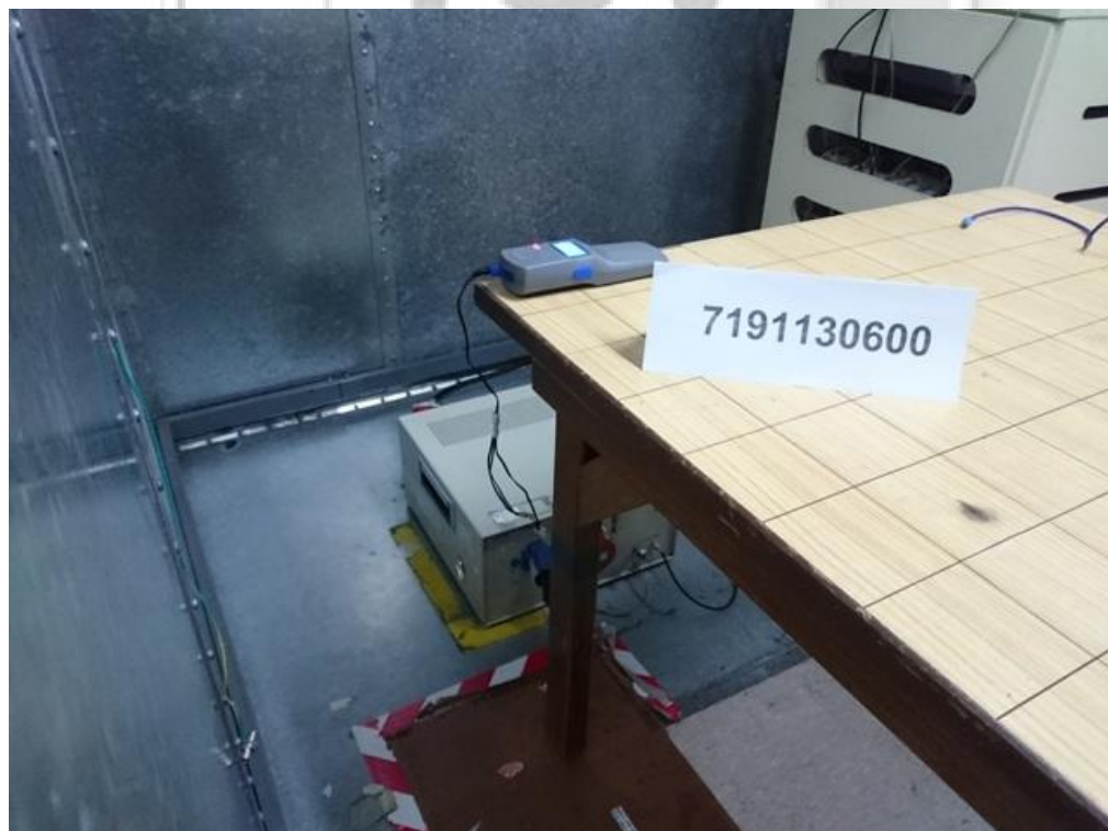
Conducted Emissions Test Setup (Rear View)
