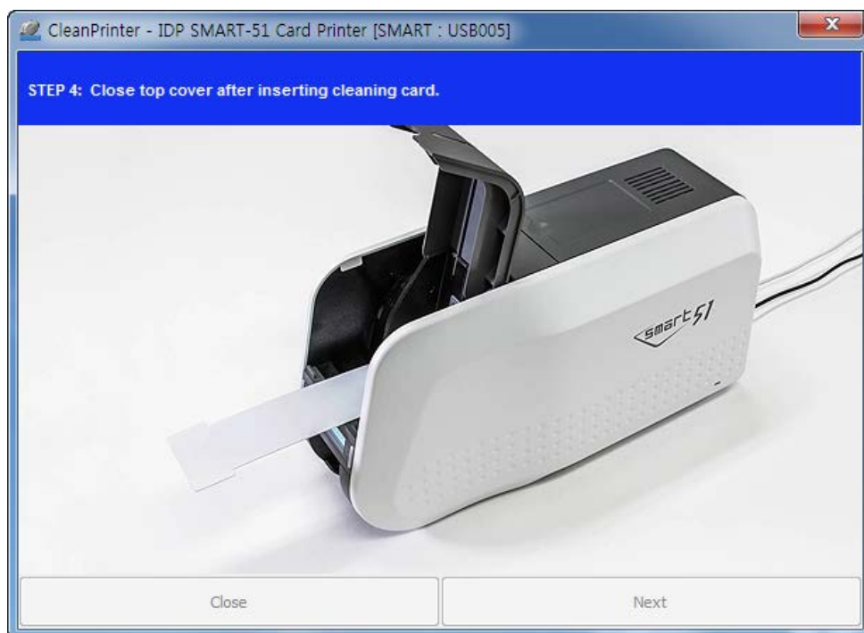
Figure 107 Printer cleaning Step 4
