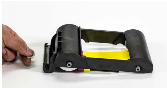
Figure 18 Peeling the protective wrapper
