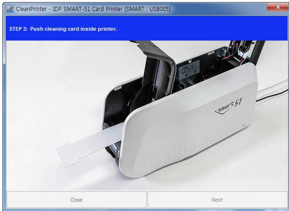
Figure 106 Printer cleaning Step 3
