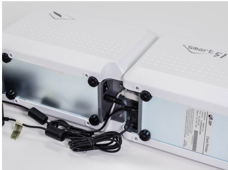
Figure 11 SMART-51L Connection of powers and USB cable - 1
