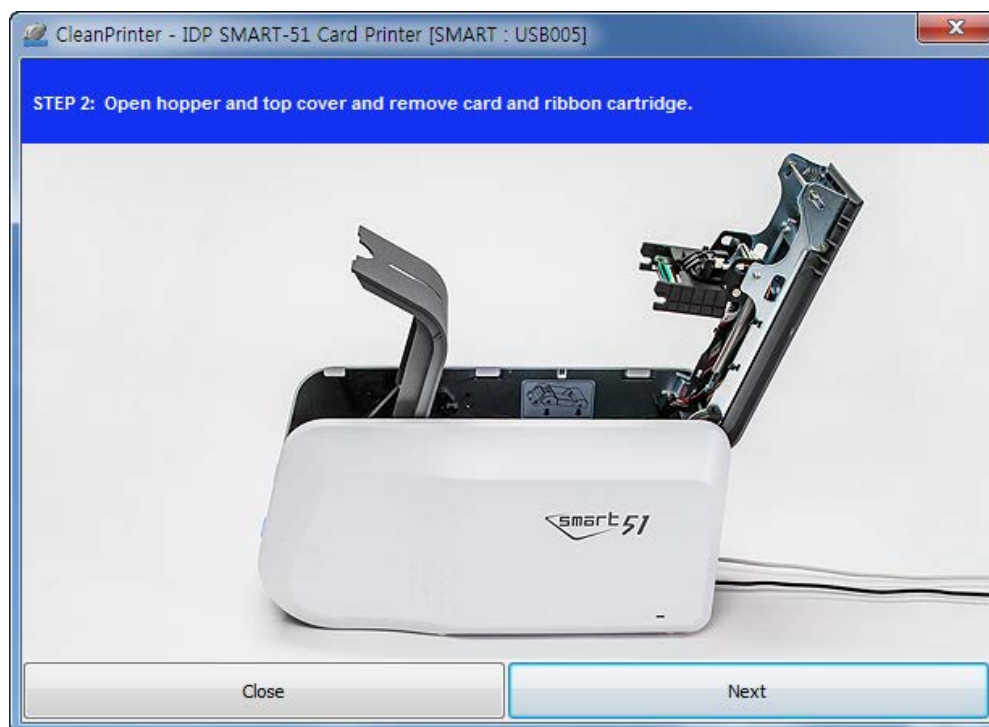
Figure 105 Printer cleaning Step 2
