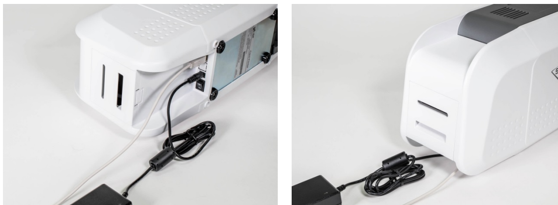
Figure 10 SMART-51D Connection of power and USB cable
