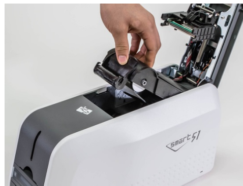
Figure 19 Installing the ribbon cartridge
