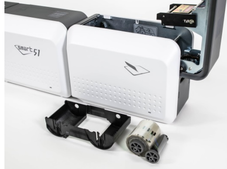
Figure 21 Take out the film cartridge
