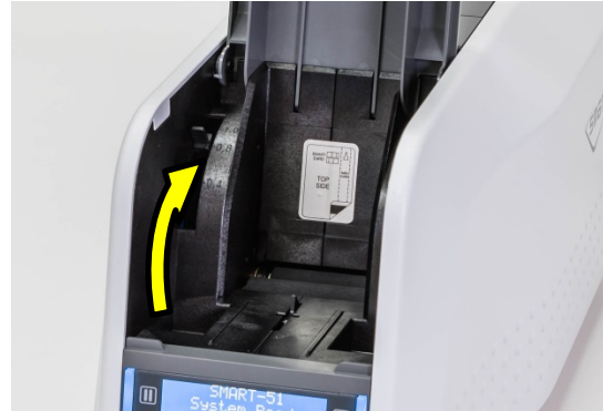
Figure 24 Adjusting the card thickness lever
