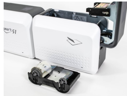
Figure 22 Loading the laminating film
