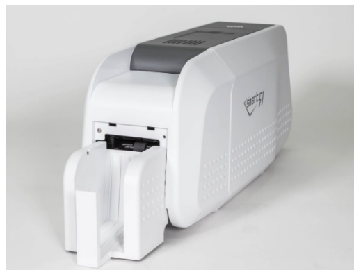
Figure 34 SMART-51D installation of Rear Stacker
