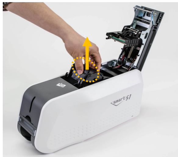
Figure 14 Take out the ribbon cartridge
