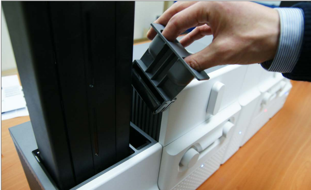
Figure 32 Installation of disposable cleaning roller holder
