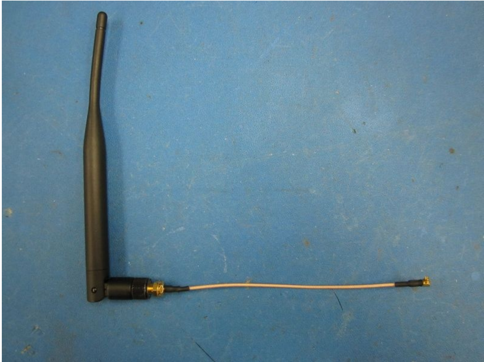
5dBi Omni antenna and MMCX -> reverse SMA cable
