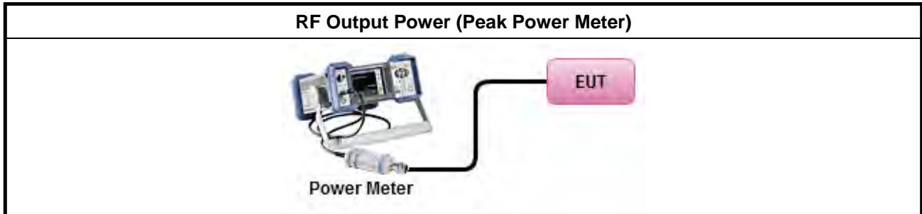
3.5.5 Test Result of Maximum Peak Conducted Output Power
