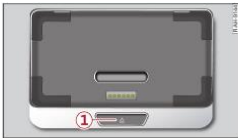
Fig. 2 Centre armrest (rear): Rear Seat Remote holder
