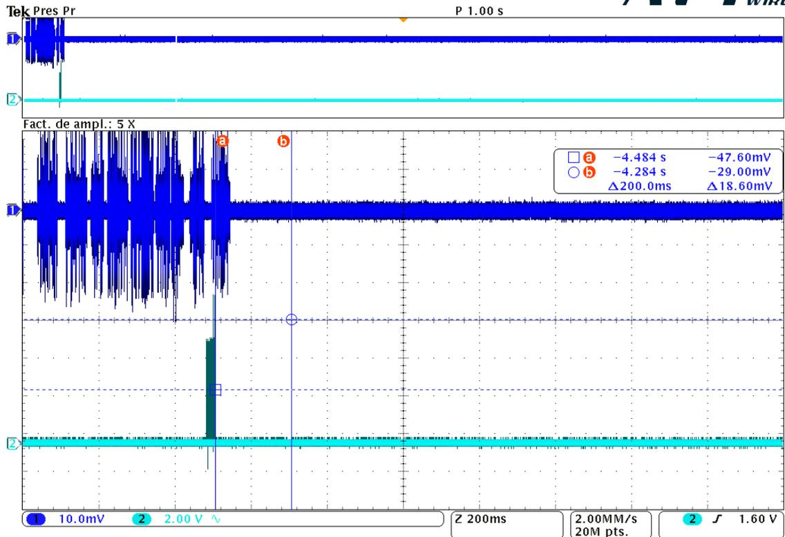
This plot provides a zoom-in to show the 200 ms time interval after the radar burst.
