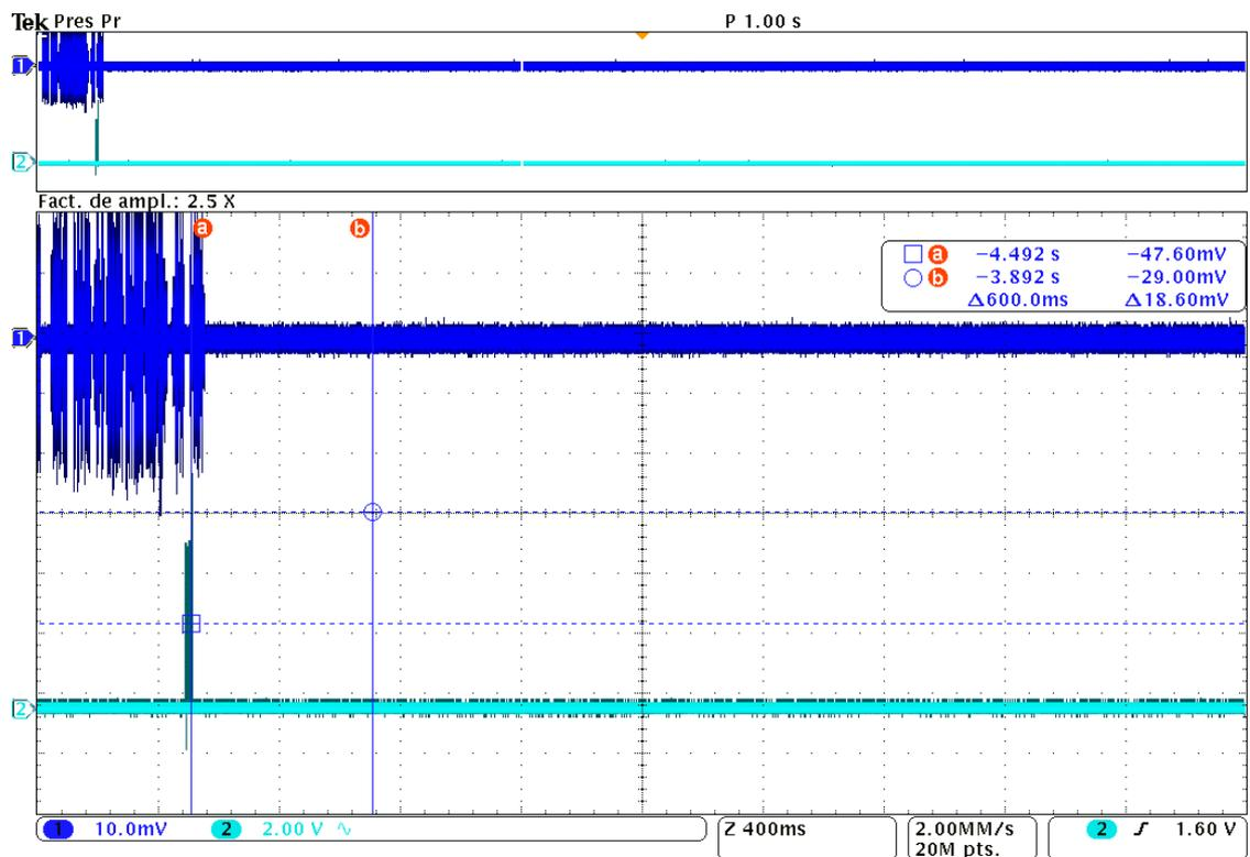
This plot provides a zoom-in to show the 600 ms time interval after the radar burst. This shows that there were not any transmissions after 200 ms following the radar burst.
