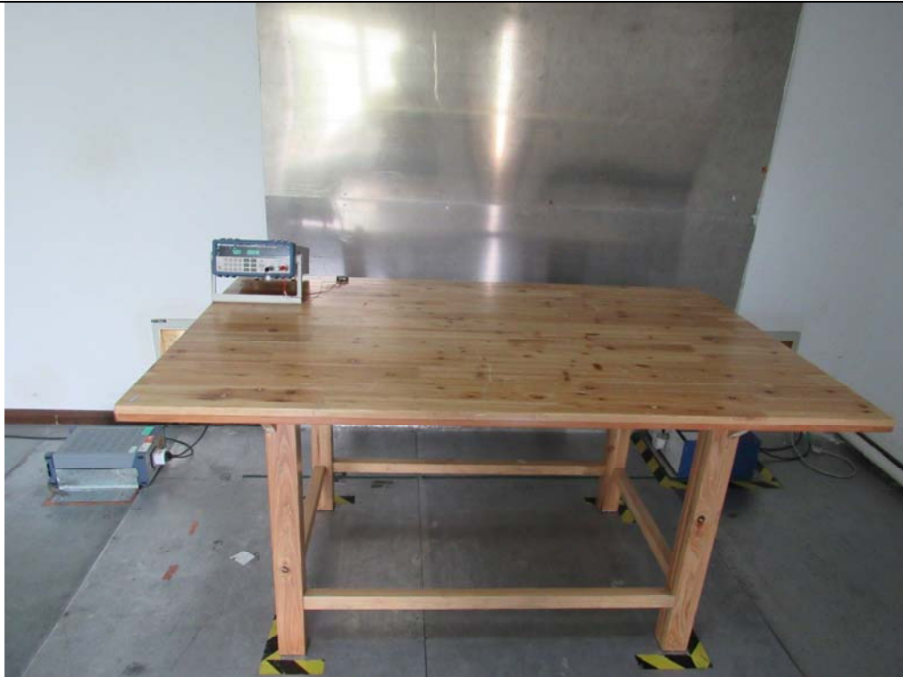
Conducted Emissions Setup Front View
