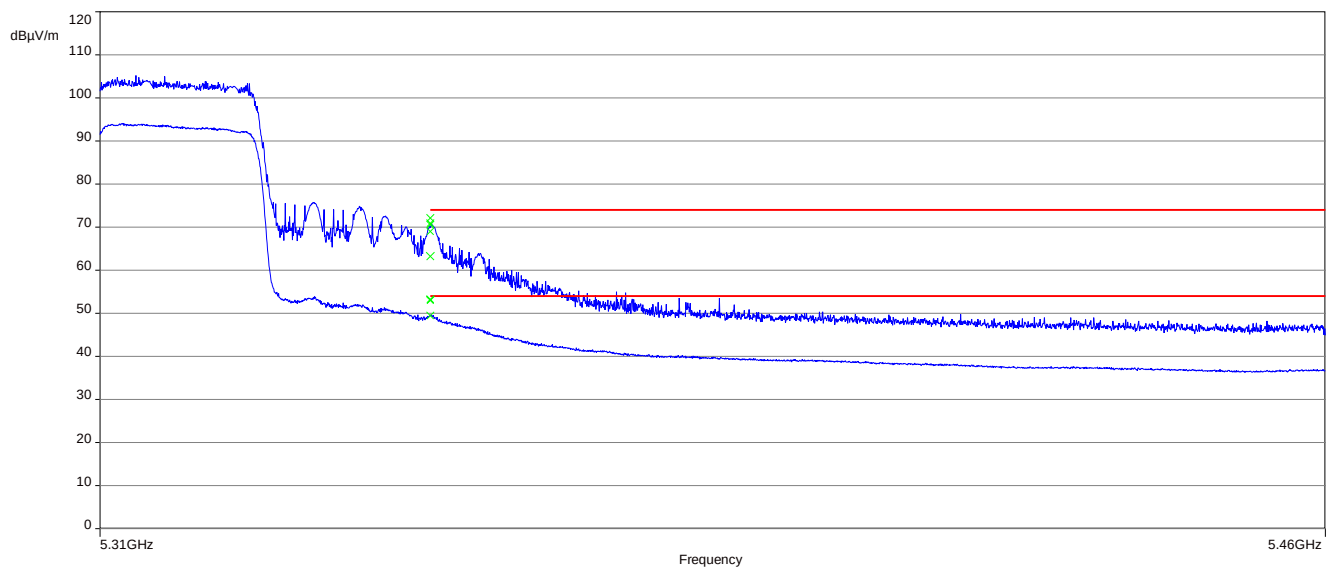
Plot 20: upper band edge; U-NII-2A; highest channel; ax40-mode
