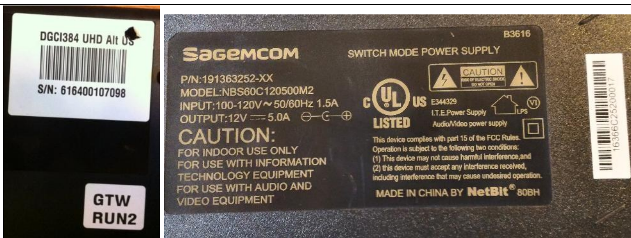
Power supply n° 1
