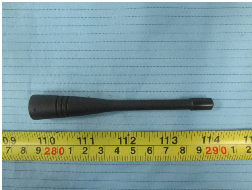
EUT – 900MHz Antenna View
