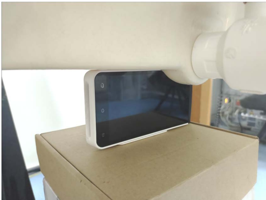
Body Left Setup Photo (0mm)
