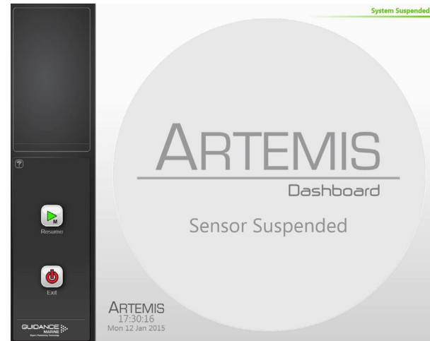
Dashboard screen with local station suspended
