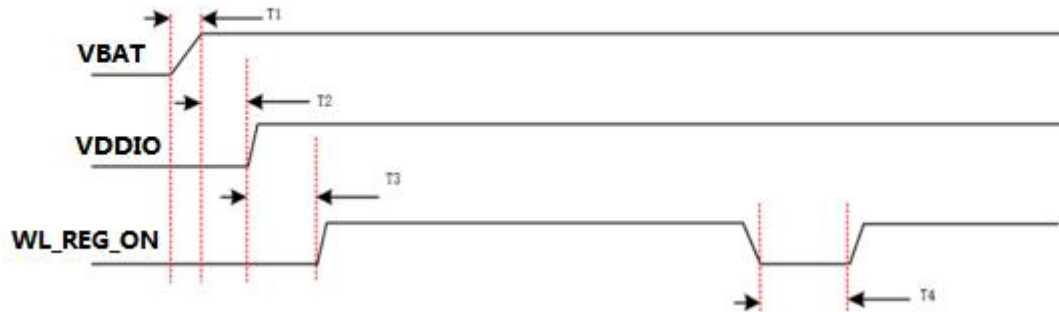
Figure 4. Power-up and Power-down Timing of SW6621-44B1
