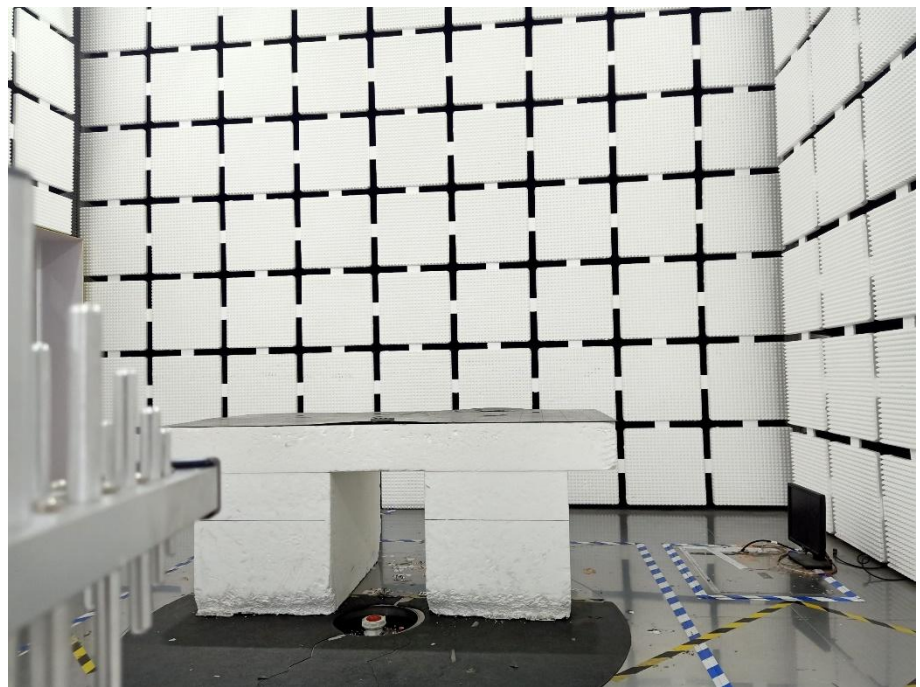
Radiation Emission Test Setup (30MHz to 1GHz)
