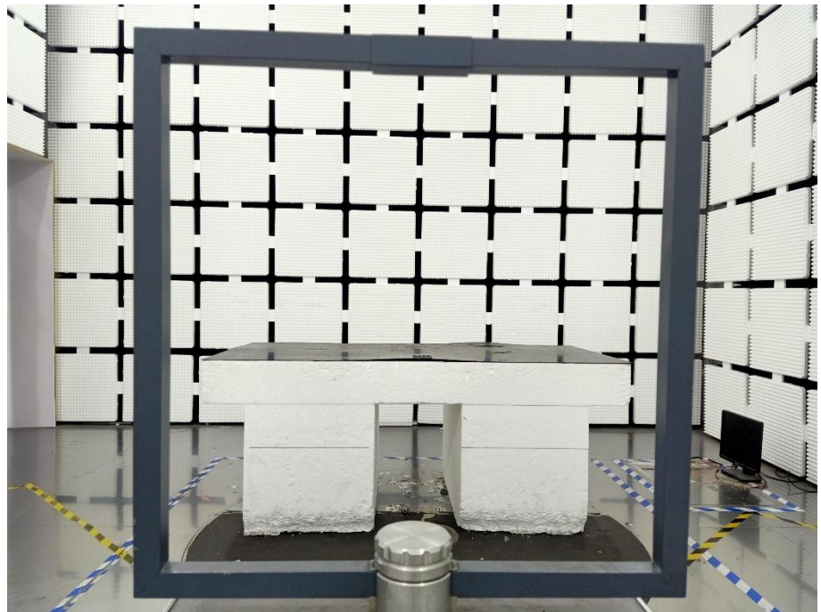
Radiation Emission Test Setup (Below 30MHz)
