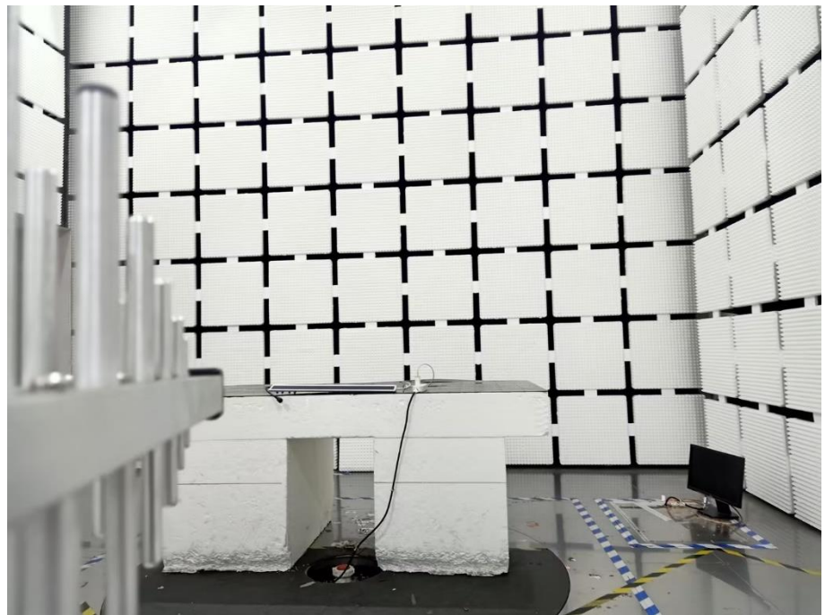
Radiation Emission Test Setup (30MHz to 1GHz)
