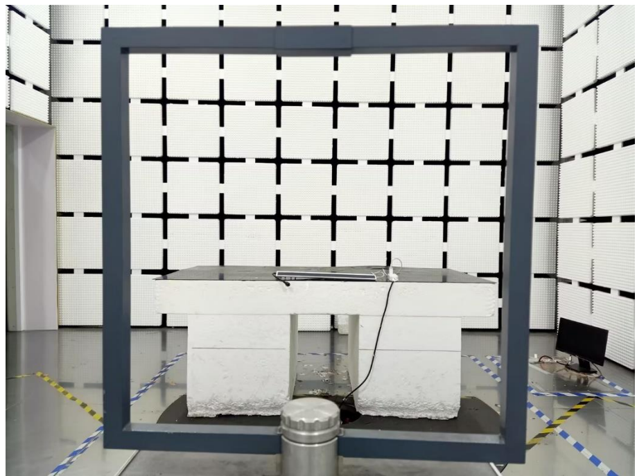
Radiation Emission Test Setup (Below 30MHz)
