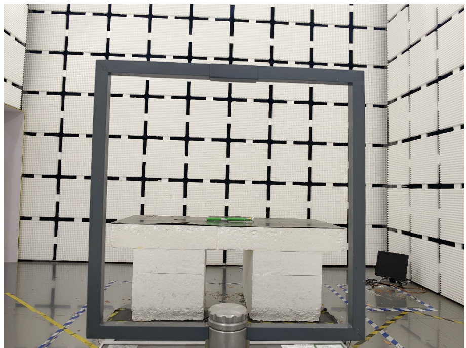
Radiation Emission Test Setup (Below 30MHz)
