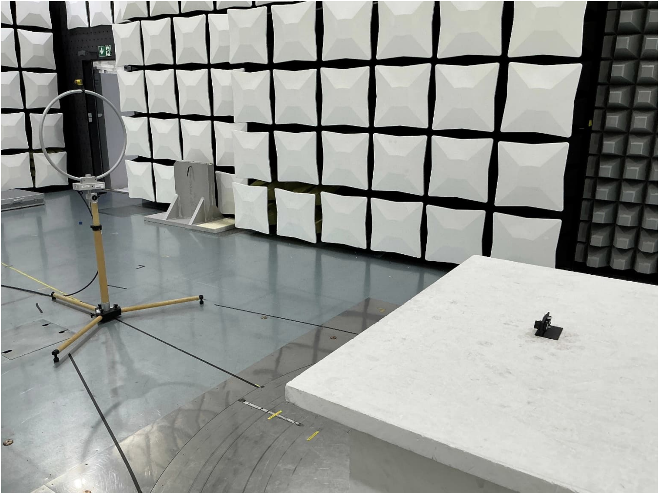
Preliminary measurement H-Field 9 kHz to 30 MHz in SAC
