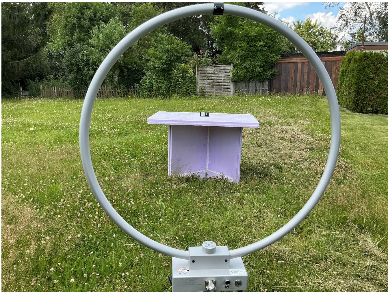
Final measurement H-Field 9 kHz to 30 MHz outdoor
