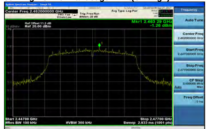
802.11n HT20 PSD for Bandedge Limit(CH-Low)
