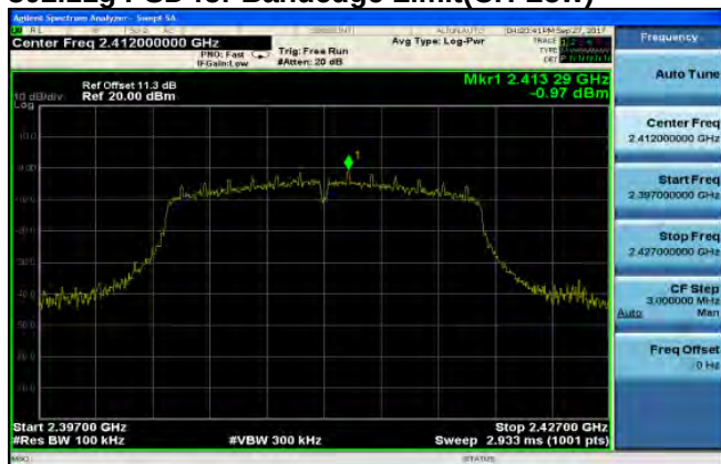
802.11g PSD for Bandedge Limit(CH-Low)
