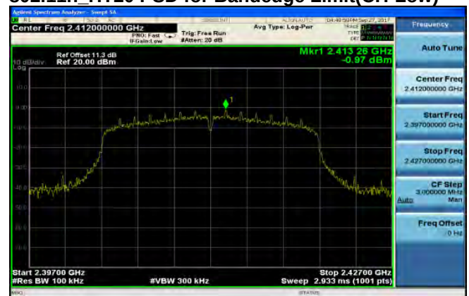
802.11n HT20 PSD for Bandedge Limit(CH-High)
