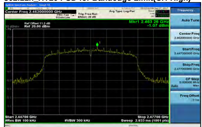
802.11n HT20 PSD for Bandedge Limit(CH-High)
