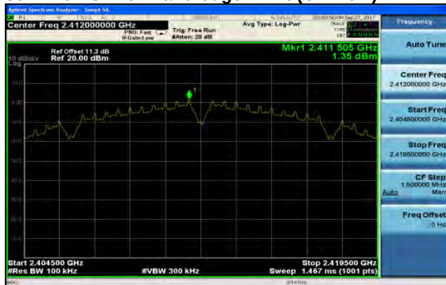
802.11b PSD for Bandedge Limit(CH-High)
