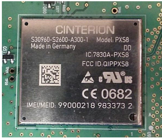
EUT – WWAN Radio with Shielding
