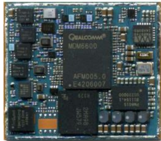
EUT – WWAN Radio without Shielding
