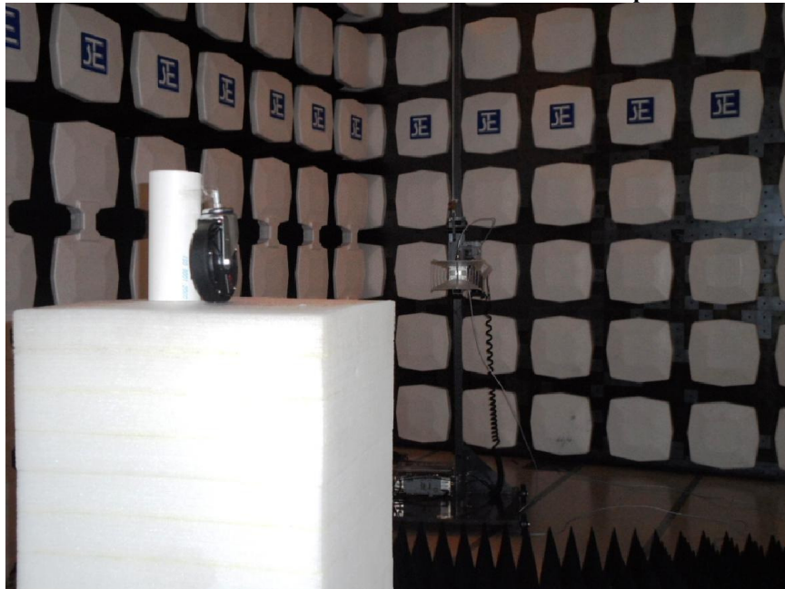
Measurement of Radiated Emission Test Set Up
