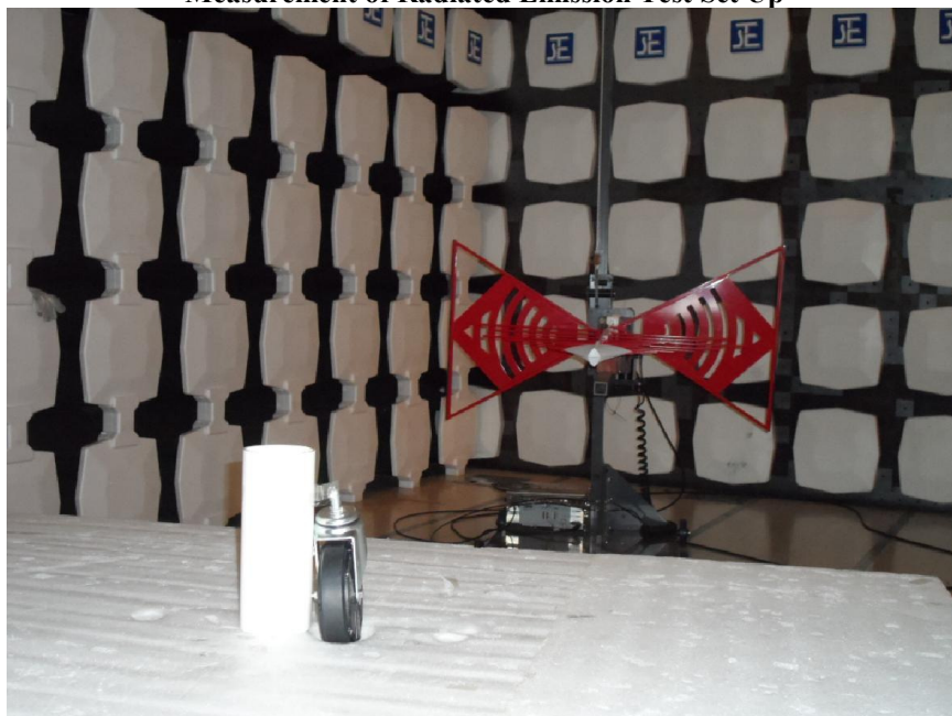
Measurement of Radiated Emission Test Set Up
