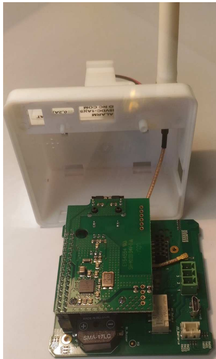
Back face with ethernet card
