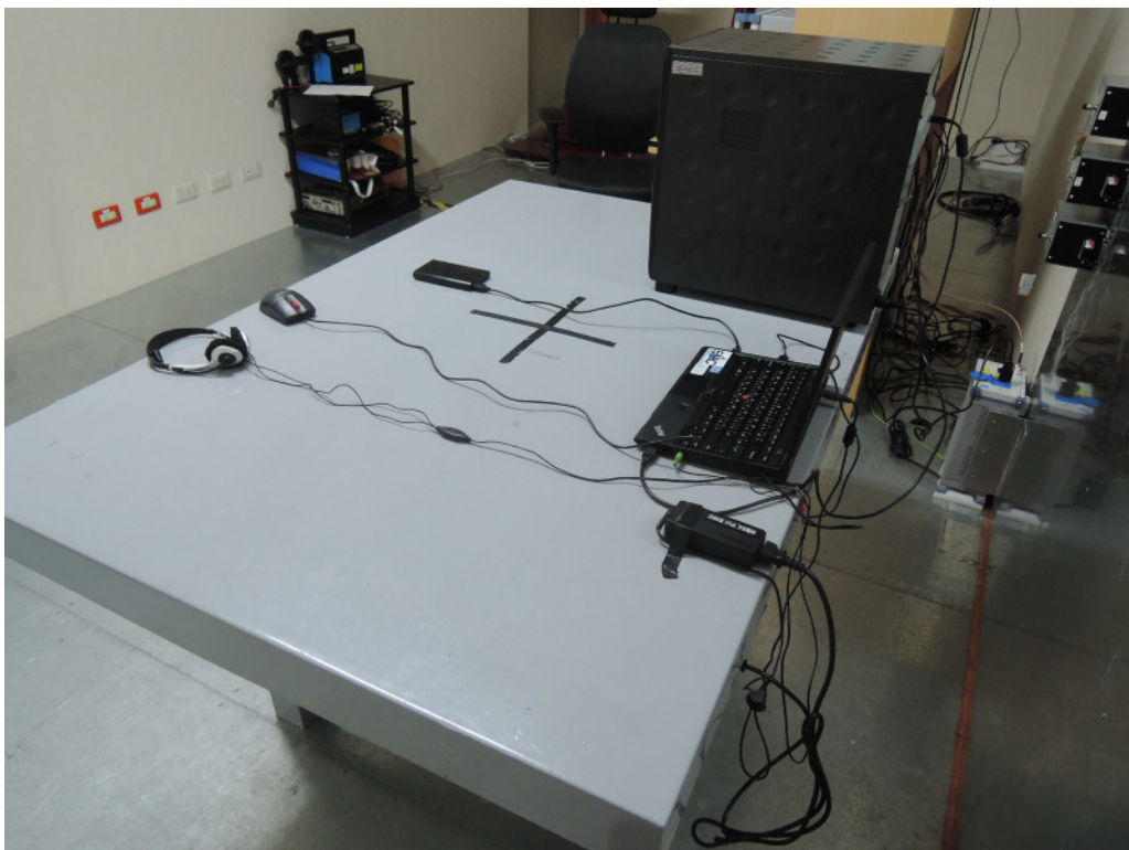
Photograph 6: Set-up for for Mains Conducted testing Front
