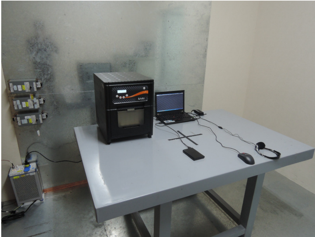
Photograph 5: Set-up for for Mains Conducted testing Back
