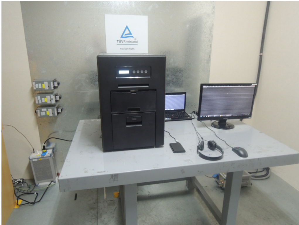
Photograph 7: Set-up for Mains Emissions (Back View)
