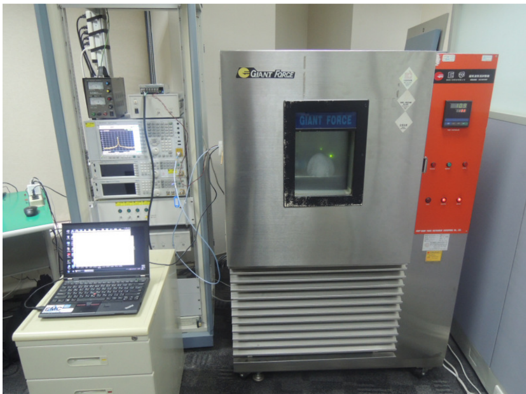
Photograph 4: Set-up for Conducted testing
