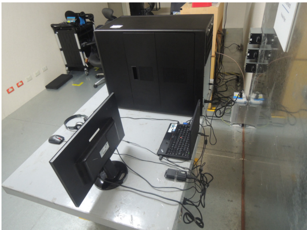
Photograph 7: Set-up for Mains Emissions (Back View)
