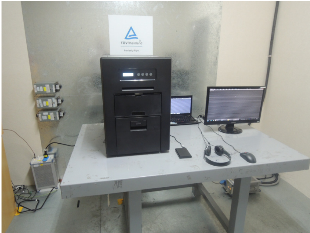
Photograph 7: Set-up for Mains Emissions (Back View)
