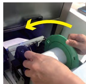
Step3. Hold onto the flange and roll it as the arrow indicated to roll out jammed paper.*
