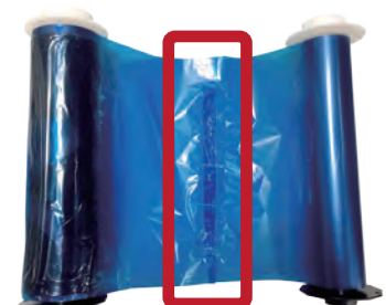
Tape the ribbon back together , and place ribbon back onto cartridge. Make sure to scroll the ribbon back onto the cartridge as tight as possible, till the broken part of the ribbon cannot be seen.
