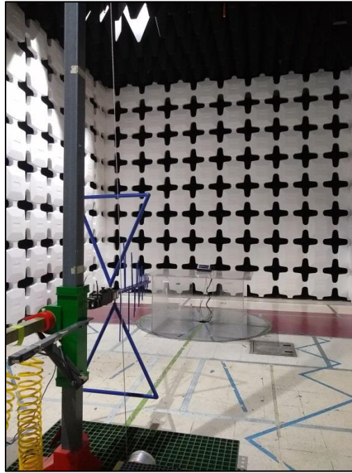
Photograph 1. Radiated Emissions, 30 MHz – 1 GHz, Test Setup
