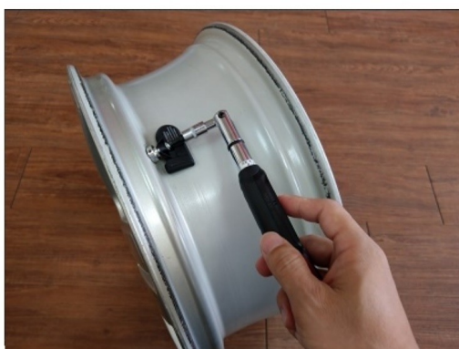
Install sensor. Adjust the sensor to fit the drop well of the wheel. Use wrench to keep stem vertical then tighten. Tighten the screw until 2.2Nm (Recommended Final Torque Setting)
