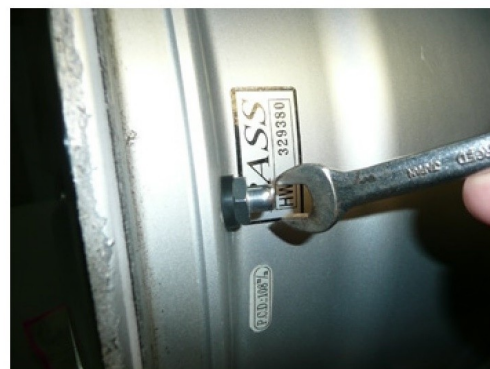
Use wrench to hold valve stem and keep vertical while
