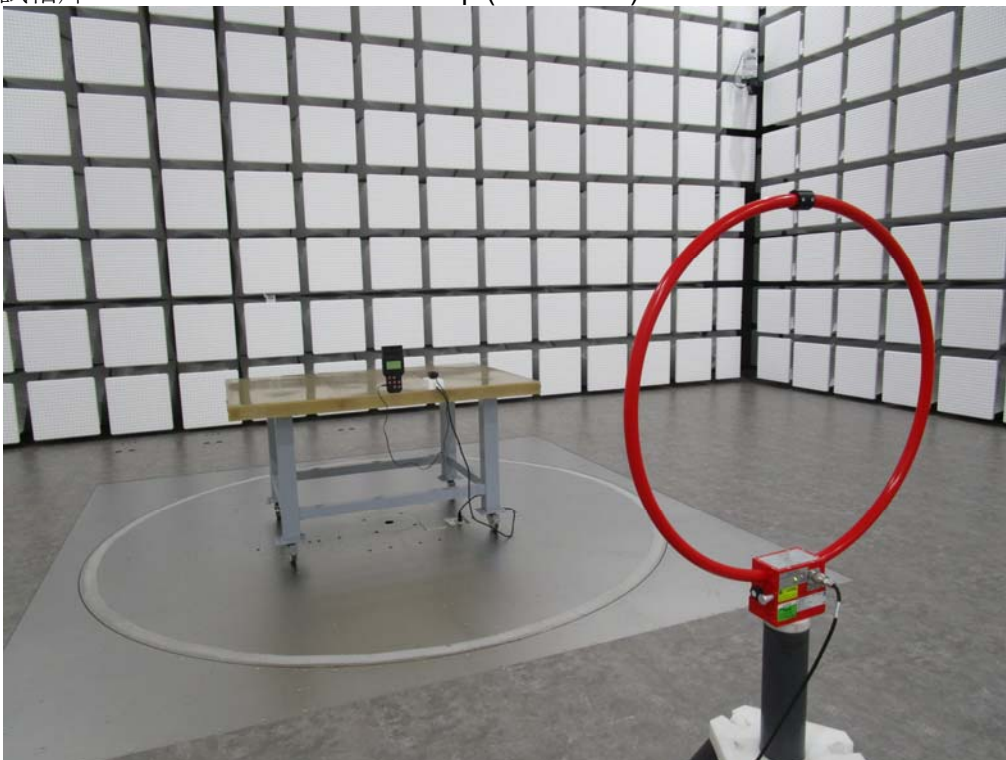
測試相片 : Back View of Test Setup (9k-30MHz)
