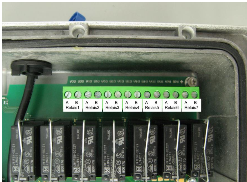
Figure 9: Relay terminal block B1
