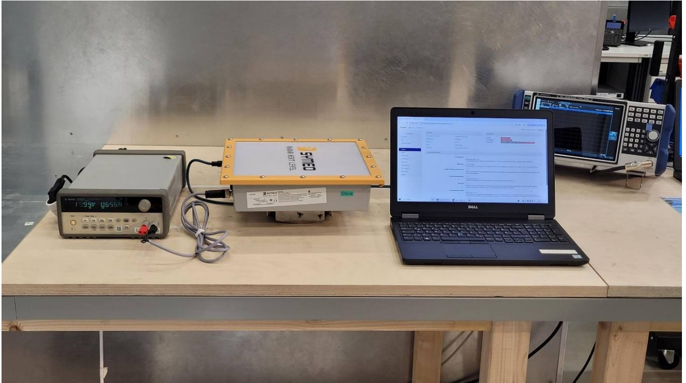
Photo No. 46 Test Setup AC conducted emissions
