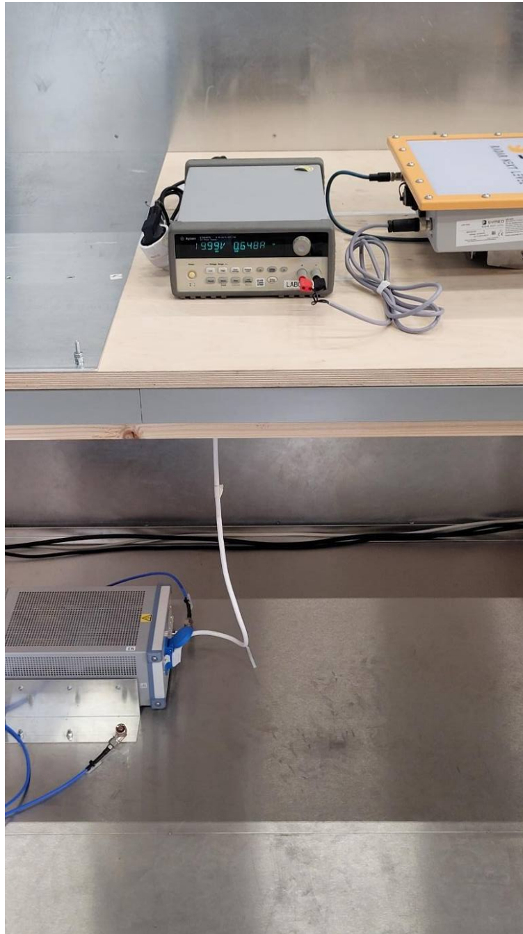
Photo No. 47 Test Setup AC conducted emissions
